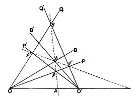
Let OB, OP, OQ cut O'B', O'P', O'Q' in the points b, p, q respectively; and let bp cut OO' in A. Then because the pencil  $O\{AB, PQ\}$  is harmonic, OQ must cut the line Ab in the point which is the conjugate of p with respect to A, b. Similarly O'Q' must cut Ab in the same point. Hence q the point of intersection of OQ, and O'Q', must lie on Ab. That is, the points p, b, q are collinear.
